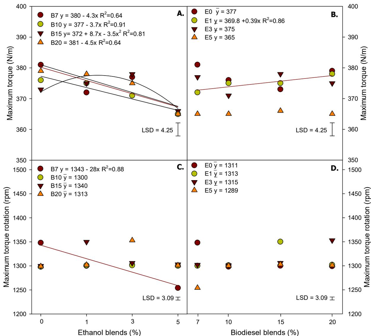
FIGURE 3. Regression analysis for maximum torque (A and B) and maximum torque rotation (C and D) of biodiesel and ethanol blends.
