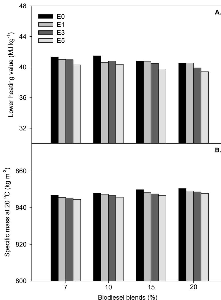
FIGURE 1. Lower heating value and specific mass of biodiesel and ethanol blends.
