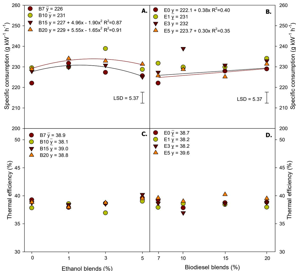
FIGURE 4. Regression analysis for specific consumption (A and B) and thermal efficiency (C and D) of biodiesel and ethanol blends.
