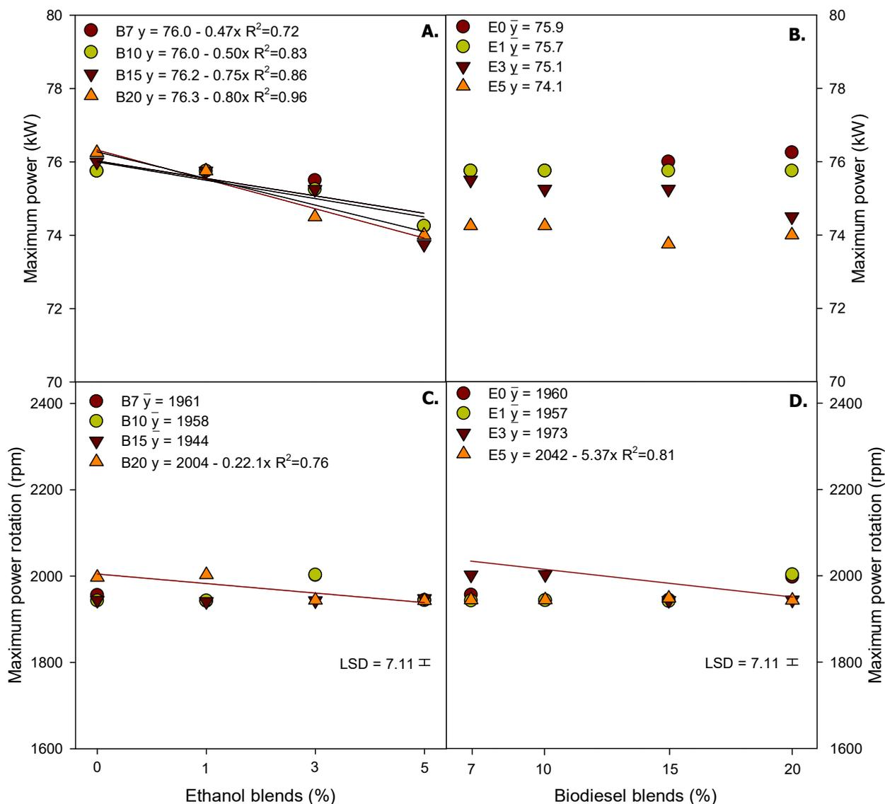
FIGURE 2. Regression analysis for maximum power (A and B) and maximum power rotation (C and D) of biodiesel and ethanol blends.
