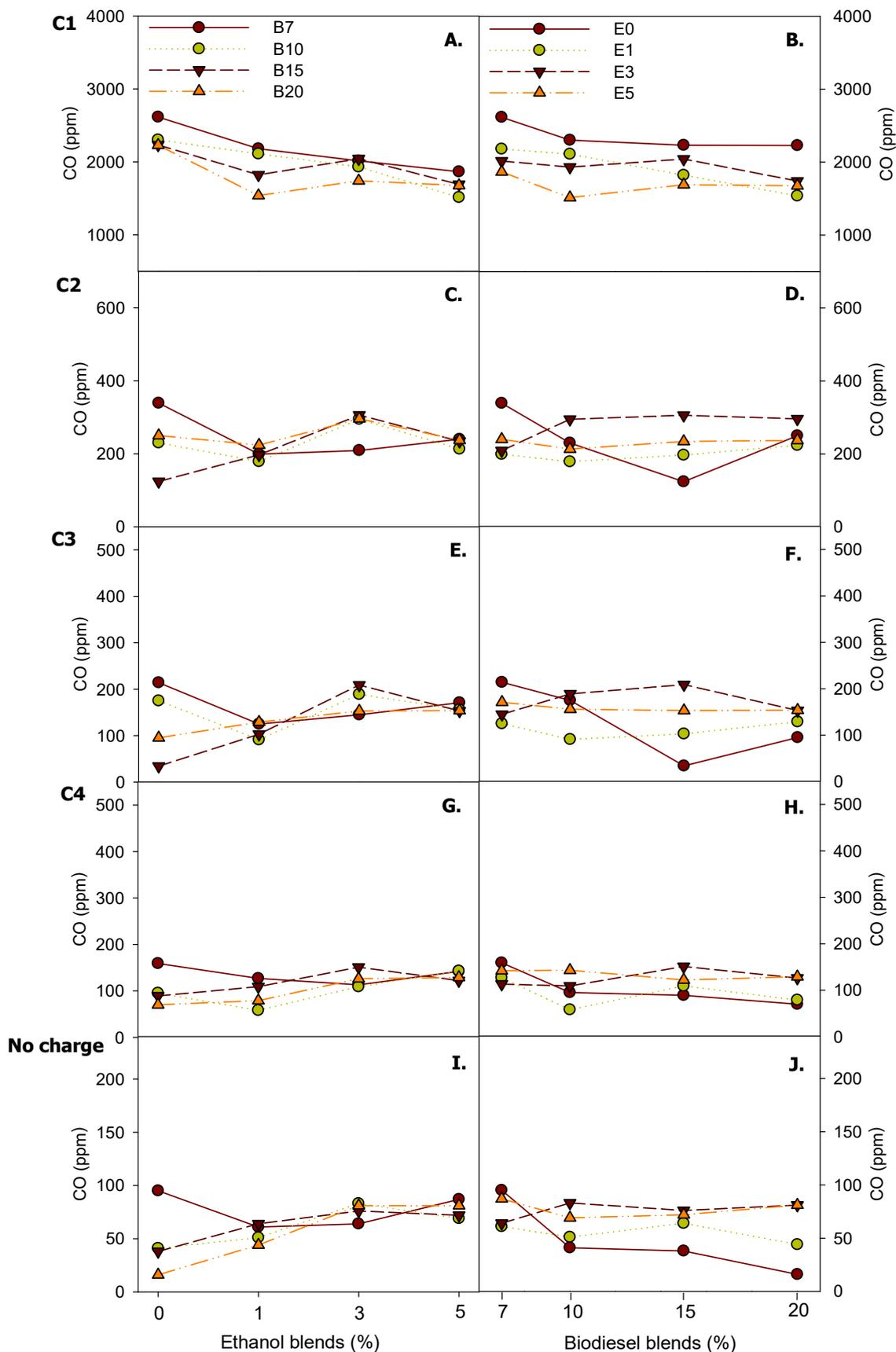
FIGURE 6. CO emissions in biodiesel and ethanol blends at different engine loads (A-J).
