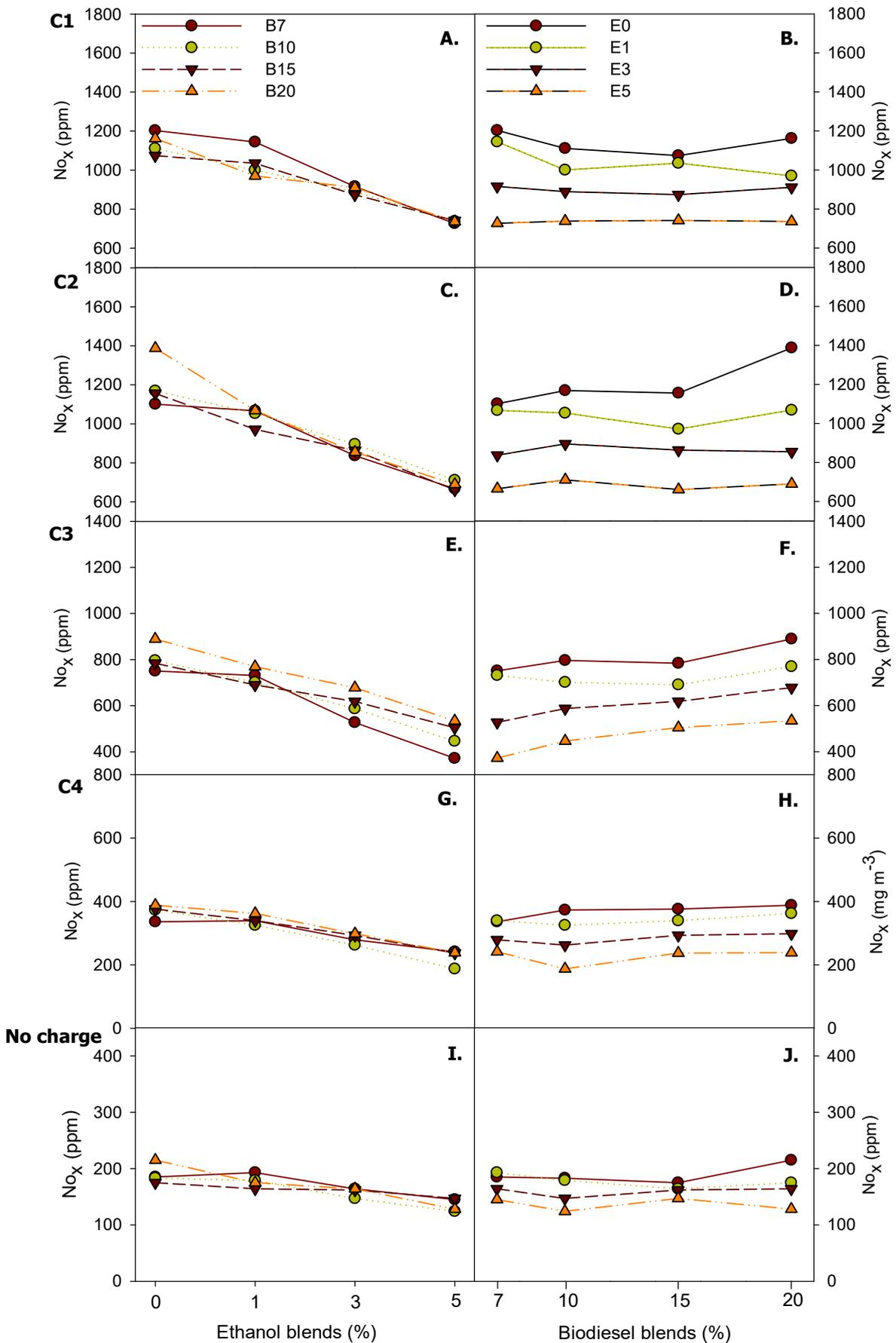
FIGURE 5. NO<sub>x</sub> emissions in biodiesel and ethanol blends at different engine loads (A-J).
