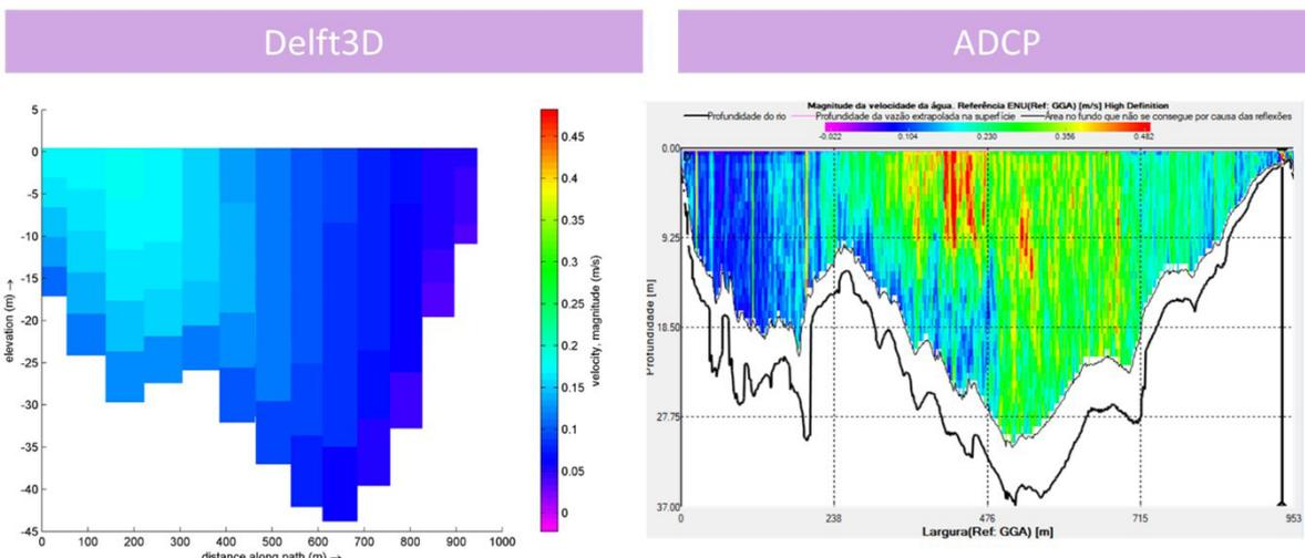
Figure A9. Transect illustrating magnitude of horizontal velocities - Lower flow: 3,599 m<sup>3</sup>/s – 09<sup>th</sup> Aug 2016.
