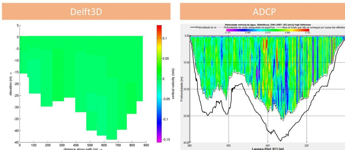
Figure A6. Transect illustrating magnitude of vertical velocities - Low flow: 6,808 m<sup>3</sup>/s - 16<sup>th</sup> Aug 2018.
