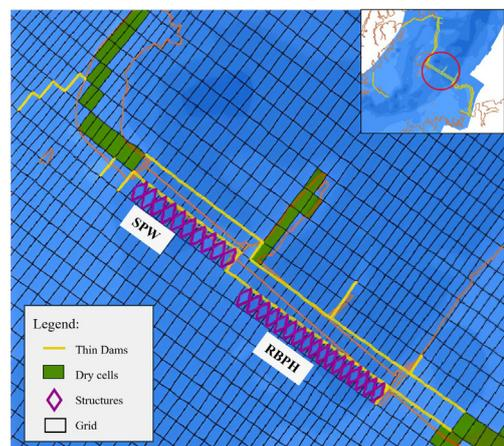
**Figure 5.** Representation of the dam structures implemented in the Delft3D model. Zoomed image in SPW and RBPB. Scale: 1:10,000.
