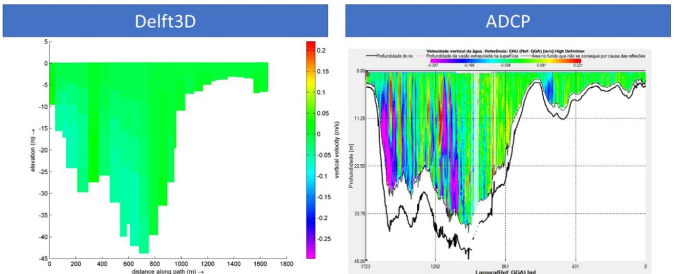
Figure 11. Transect illustrating magnitude of vertical velocities - High flow - 25<sup>th</sup> Feb 2019.
