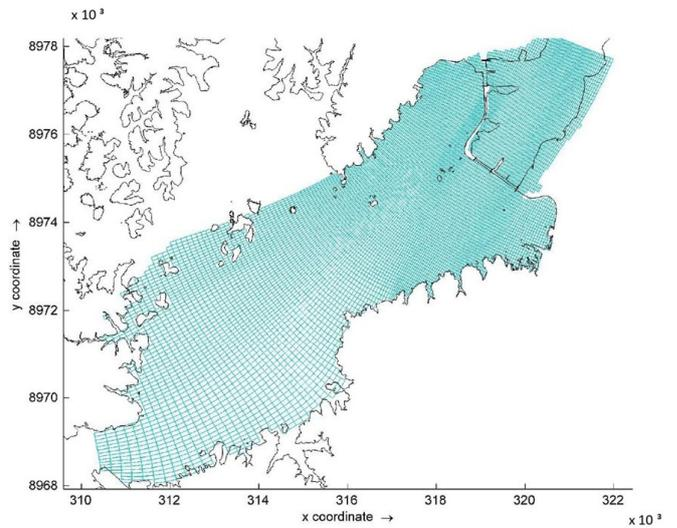
**Figure 3.** Computational Mesh – Planar view.
