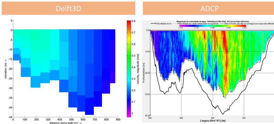
Figure A5. Transect illustrating magnitude of horizontal velocities - Low flow: 6,808 m<sup>3</sup>/s - 16<sup>th</sup> Aug 2018.
