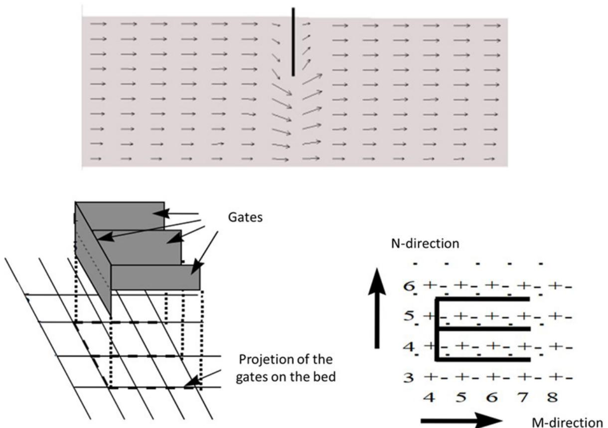
Figure 7. Illustrative example of the “3D gate” structure in a cross section (Deltares, 2023a).
