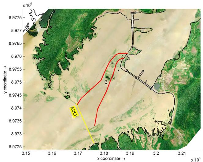
Figure 8. Schematic representation of log booms positions in red and ADCP section in yellow.
