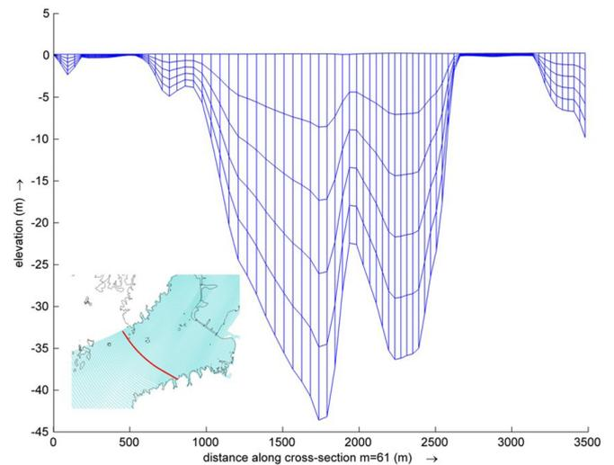
**Figure 4.** Vertical grid using sigma coordinate system in a reservoir section.
