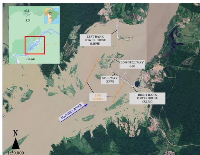
**Figure 2.** Jirau Hydroelectric Power Plant structures.
