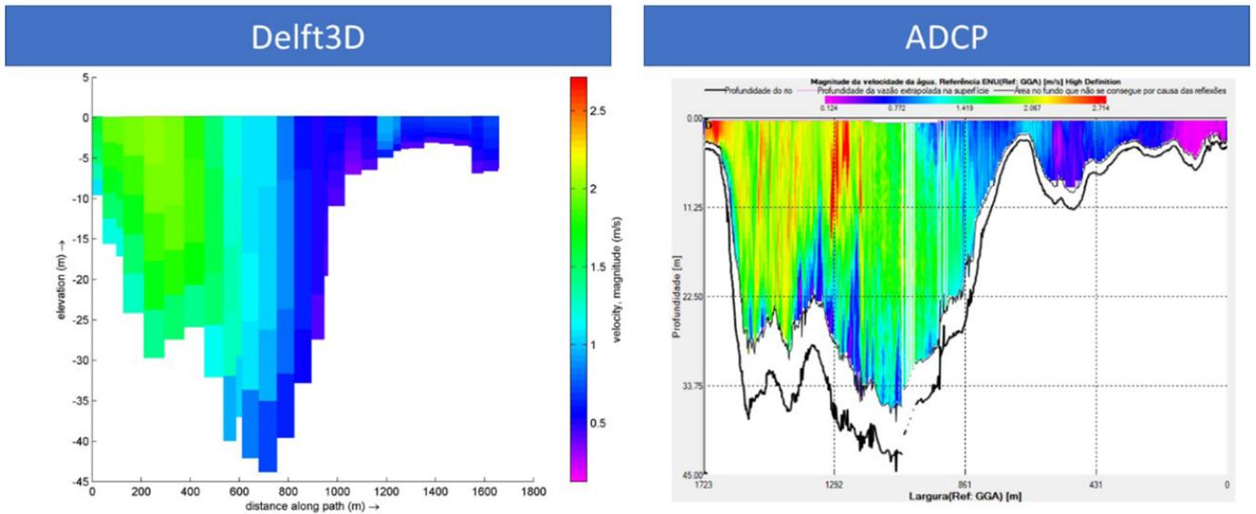
Figure 10. Transect illustrating magnitude of horizontal velocities - High flow - 25<sup>th</sup> Feb 2019.
