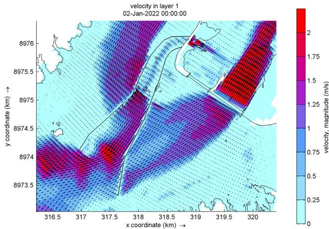
Figure 20. Velocities near the log boom for Scenario 1.
