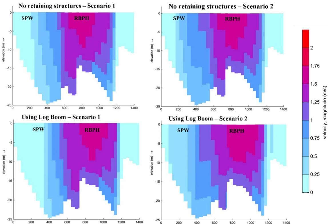
Figure 17. Magnitude of velocities on the right bank of the Jirau HPP reservoir for each scenario.
