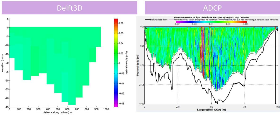
Figure A10. Transect illustrating magnitude of vertical velocities - Lower flow: 3,599 m<sup>3</sup>/s – 09<sup>th</sup> Aug 2016.
