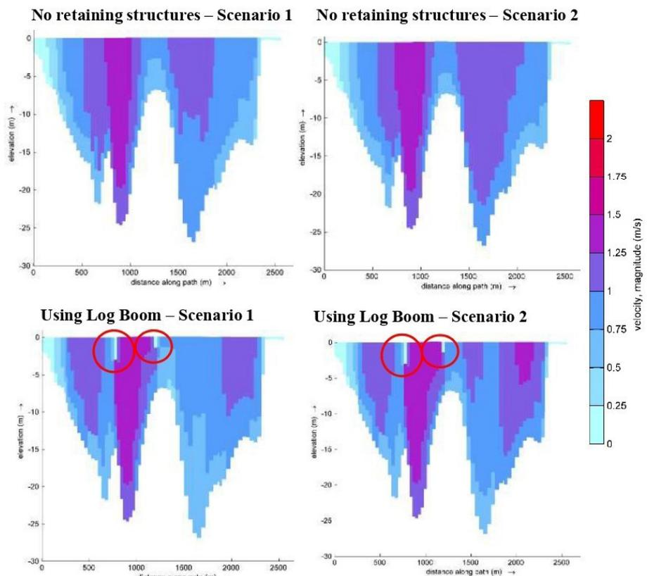
Figure 19. Magnitude of velocities in the section named S11 through the log boom.
