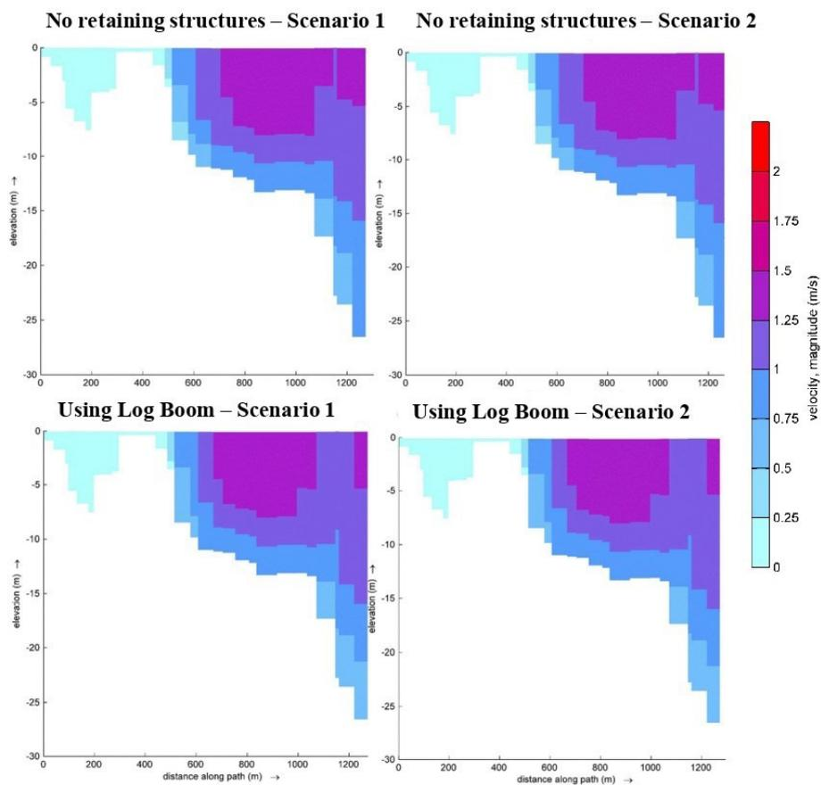
Figure 18. Magnitude of velocities at transect on the left bank of the Jirau HPP reservoir for each scenario.
