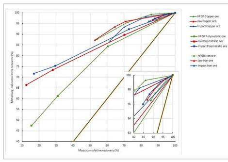
Figure 4 - Metallurgical recovery vs. Mass recovery - fraction - 6.35 + 3.35 mm.
