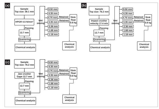
Figure 1 – Test flowchart. HPGR (a), Impact crusher (b), Jaw crusher (c).
