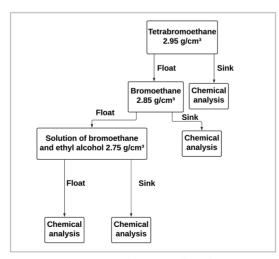
Figure 2 - Sink-float test flowchart.
