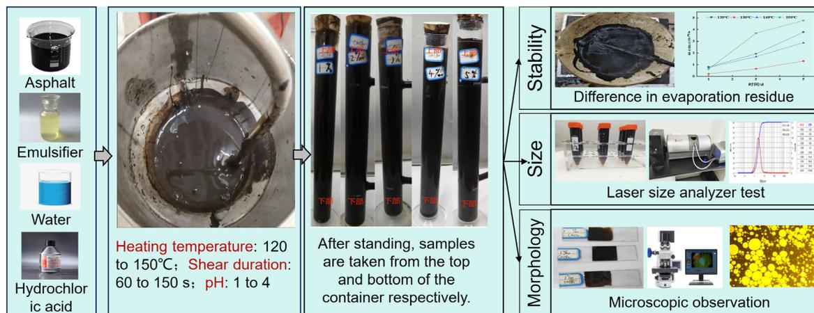
Figure 2: Experimental procedure.
