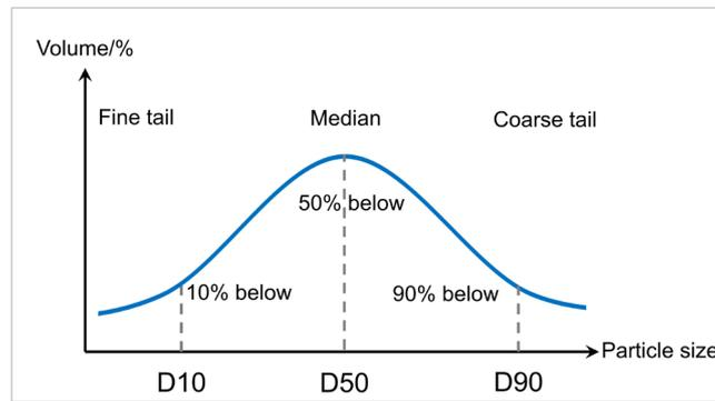
Figure 1: Physical significance of D10, D50, and D90.
